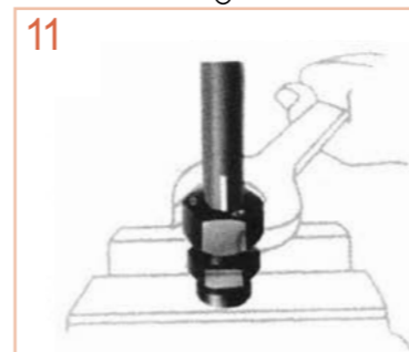
11 tighten up nut with 1 1/2 turn. (tube should not turn together)
