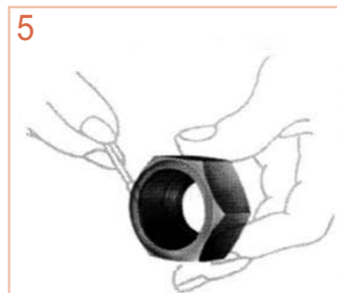
5 apply the oil to the nut thread
