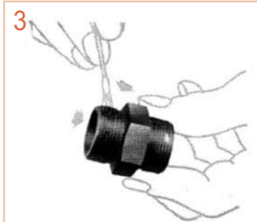
3 apply the oil to the inside and outside of Body.
