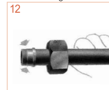
12 sleeve should turn freely on the tube.
