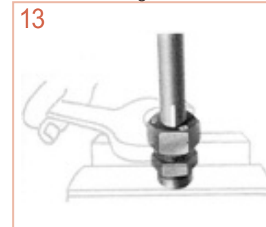
13 Tighten the NUT 1/4 turn from the sharp torque rize point.
