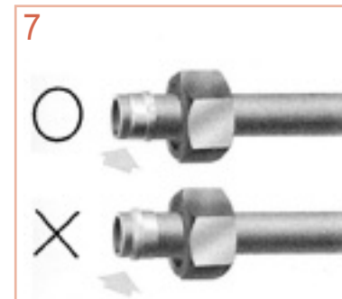
7 check the direction of sleeve.
