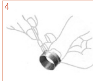
4 apply the oil to the sleeve.
