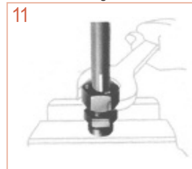
11 tighten up nut with 1 1/2 turn. (tube should not turn together)
