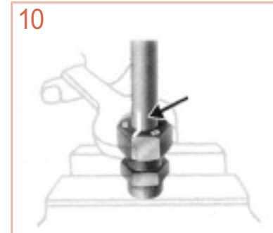
10 setting up the point before tighten up the nut.
