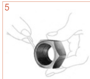
5 apply the oil to the nut thread
