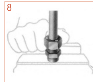
8 assemble the NUT with hand.
